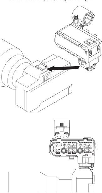
**3.** Using the lock lever (28) or the tightening dial (29), attach this unit to the connected device securely.
