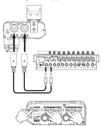
When connecting a mixer or other line level equipment, use XLR or TRS cables to connect it to this unit, and set the INPUT 1 (4) and INPUT 2 (7) switches to "LINE".
