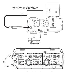
When connecting a stereo lapel mic, for example, connect it to the INPUT 3 jack (②), and set the SELECT switch (②) to "IN 3".
