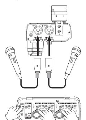
When connecting a mic to the INPUT 2 jack (②) set the SELECT switch (②) to "IN 1+2" and set the INPUT 2 switch (⑦) according to the type of mic connected.
