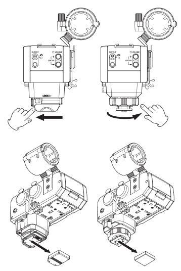
2. With the unit oriented correctly, mount the connector part to the camera accessory shoe, sliding it all the way in.
