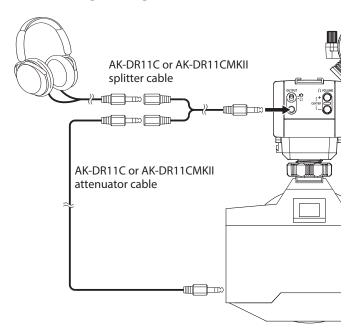
A splitter cable is necessary to monitor analog audio with a CA-XLR2d-AN.
