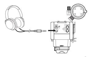
To monitor analog audio signals, set the OUTPUT switch  $(\P)$  to  $\Omega$ , and connect headphones or an earphone, for example, to the OUTPUT jack  $(\P)$ . Then use the  $\Omega$  VOLUME +/- buttons  $(\P)$  to adjust the volume.
