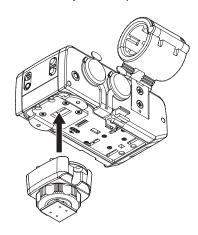
Use the 2 screws that were removed to affix the accessory shoe adapter.
