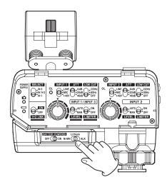
5. Set the BATTERY POWERED switch (25) to "ON" to supply power from the batteries.
