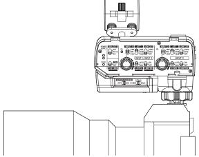
Using the tightening dial (29), attach this unit to the connected device securely.
