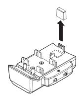
Remove the bottom connector cover from the unit and attach the battery holder to the unit.
