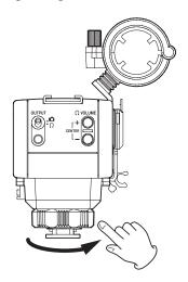
With the unit oriented correctly, mount the connector part to the camera accessory shoe, sliding it all the way in.
