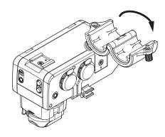
Place the mic in the holder, and close the holder while keeping the mic in place. Then, tighten the screw securely.
