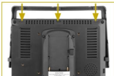
2. Gently spread the ends of the mounting frame, and press them down onto the monitor until the tabs lock into the slots on the back of the monitor.
